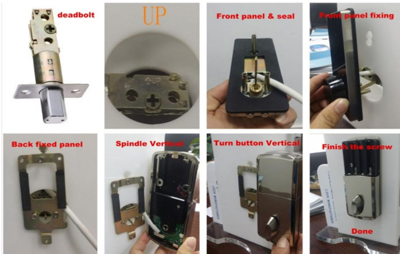
Important Note : The Long Metal Bar shown in the Third Picture on the Top Row should be in the VERTICAL position during installation (while inserting into the cross on the Dead bolt). If it is not then you wont be able to operate the lock.
